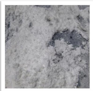
The surface of the Albasorb layer had noticeable gelling which indicated reaction with oil (left). However, the Albasorb was not completely saturated, and the oilmat was unaffected.
