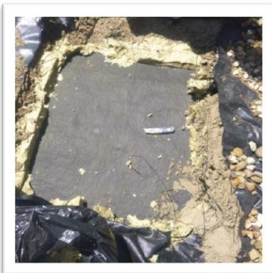
The Non woven layer also showed signs of oil penetration in this area and was cut out (left), and turned over (right).
