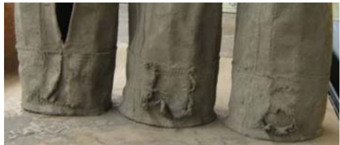
Figure 1: Re-entrained bag abrasion
