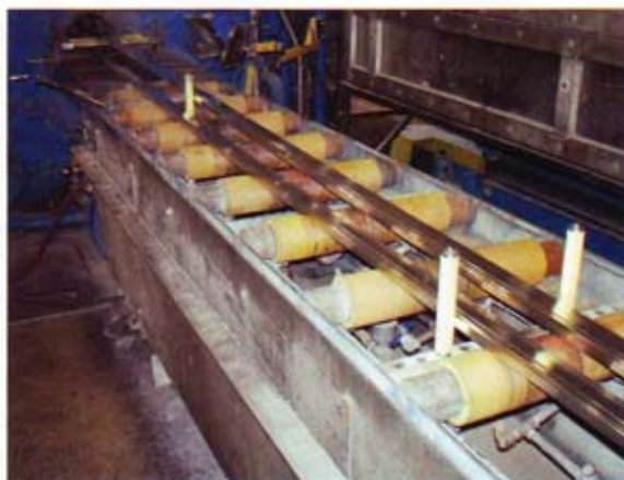
Figure 1. Slotback rollers for extrusion handling systems eliminate surface scratches or marring, enabling extrusions with a high quality surface finish.
